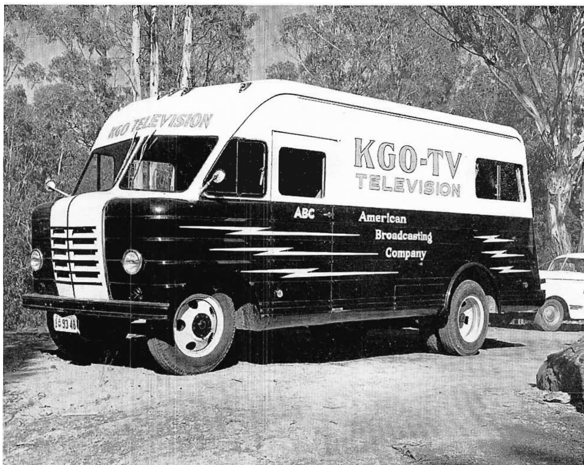
FIG. 8. View of the KGO-TV mobile unit which houses the necessary field and remote equipment. The regular crew consists of seven engineering members.
