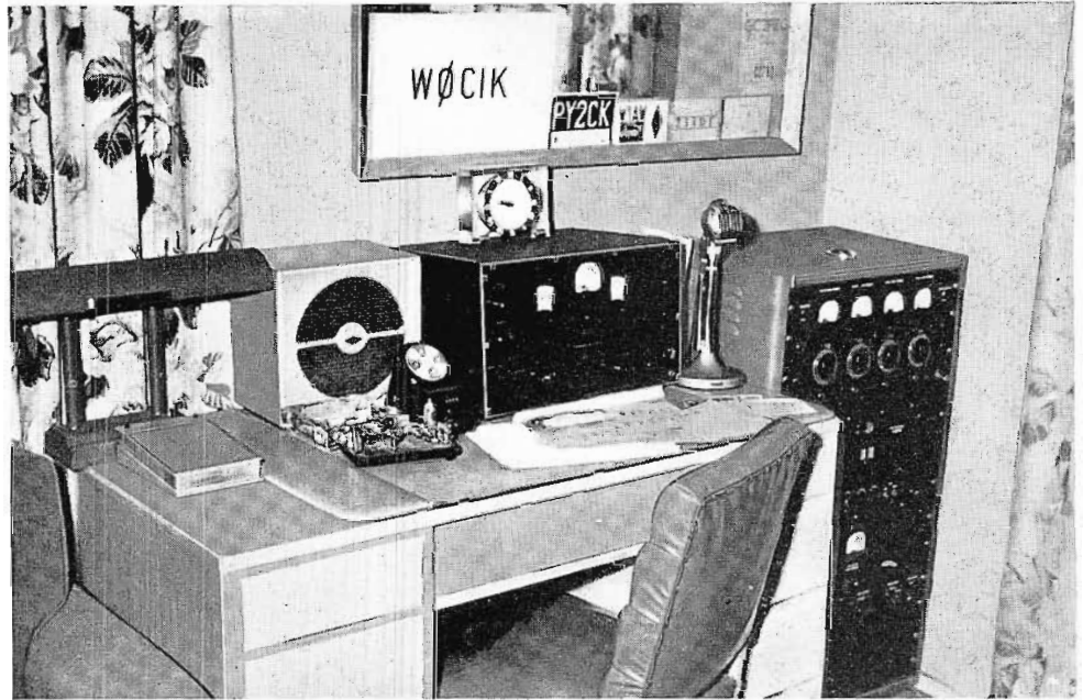
WØCIK Transmitter Room. Present transmitter runs 150 watts to pair of 24-G's.
