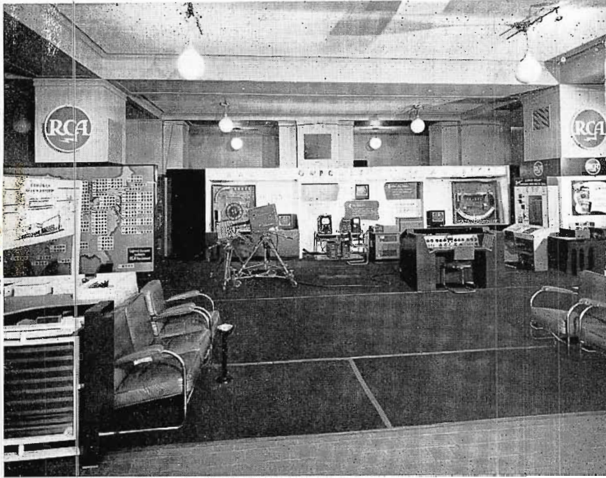
RIGHT CENTER PART of the display was devoted to a wide variety of TV studio equipment including a working setup to demonstrate the Genlock, Special Effects and the Flying Spot Camera, as well as a "Custom" TV/Audio Console.
